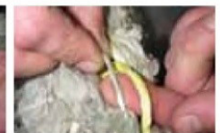
Compare surface yarns with internal yarns.
