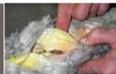
Inspect for pulled strands. Figure 2 Inspect for internal abrasion on.
